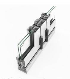
**S55 - With reinforcement column**The reinforcement column allows to manufacture glass panels up to 3 m high and 1 m wide for the S55 series.
